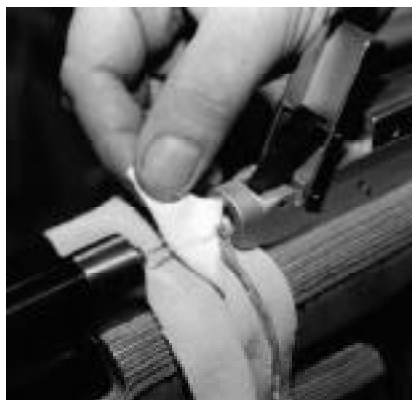
A cloth placed under the breech will keep excess solvent out of the action.
